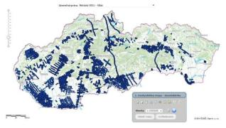
Figure 1. Map of Vertical electrical sounding (VES) measurements in Slovakia by SGIDS  $\ensuremath{\mathbb{C}}$  Map Portal (SGIDS) 2014.
