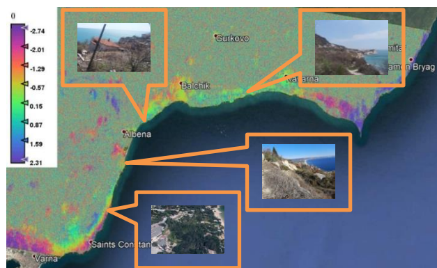
Figure 1. Interferometric image (orbit 36 ascending) for the dates 20Nov2015_11Mar2016 in the Northeast Black Sea coastal area of Bulgaria
