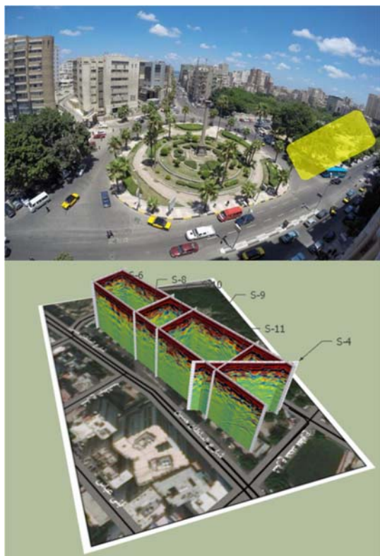
Figure 9 GPR 3D modelling at Khartoum Square at the Latin Quarter.
