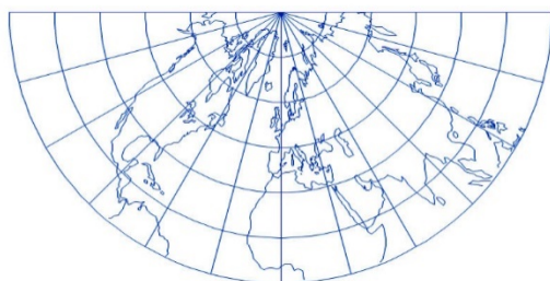
Figure 2. Conic projection equidistant along meridians, \rho = \frac{\pi}{2} - \varphi , \delta = \frac{1}{2}\lambda
