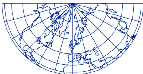
Figure 12. Conic projection with 8 standard parallels ( 10^\circ, 20^\circ, \dots, 80^\circ ). The parallels are shown with a step of 15^\circ , and the meridians with a step of 30^\circ
