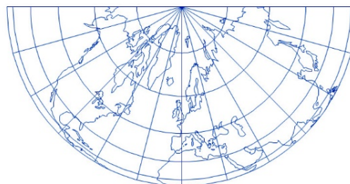
Figure 5. Conic projection equidistant along parallels, \rho = 2 \cos \varphi , \delta = \frac{1}{2}\lambda
