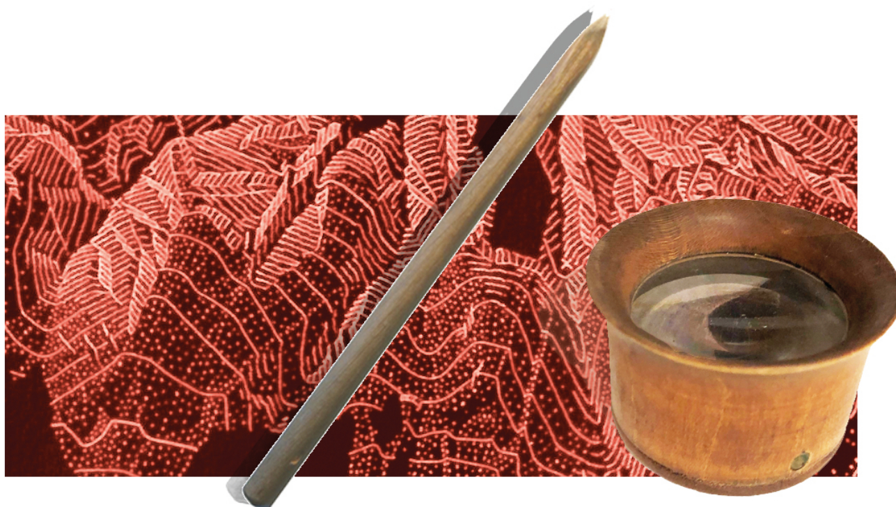
Figure 5. In the foreground, left, is a rock scribing tool (German: Dreikantnadel, a triangular ground steel needle in a wooden peg), and right, is Francis Comtesse's hand magnifier. In the background is a red, coated scribing glass plate with rock, scree and contour line scribing (negative and true-sided, drawn to the scale), which were in use at swisstopo until the year 2000. Credit: Jürg Gilgen.
