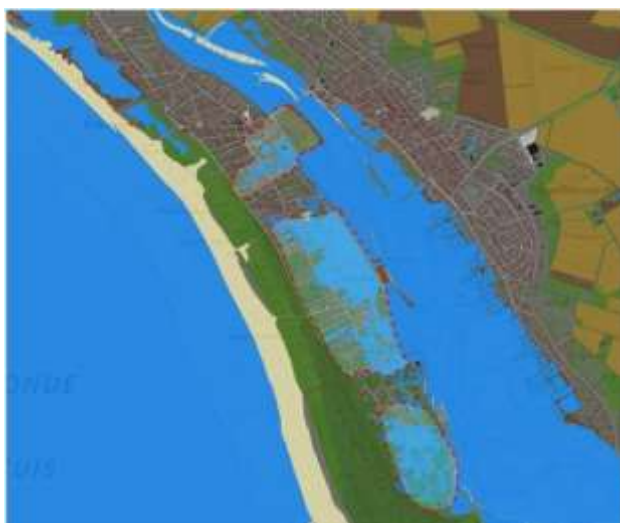
Figure 12. Minetest simulation overtopping in three breaches at La Faute sur Mer, with red dashed line superimposed on the mapping observed by SERTIT during storm Xynthia.
